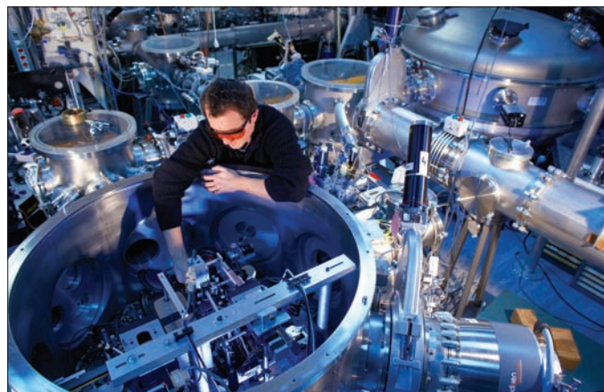
Fig. 2. The experimental chamber at the Laboratoire d'Optique Appliquée where the interaction of light with matter yields electrons, protons and X-rays. (Photos courtesy Alexis Chezière/CNRS Photothèque.)
