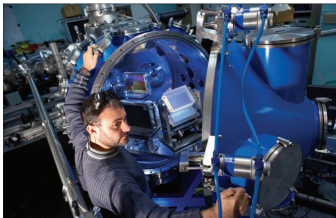
Fig. 1. The compression chamber of the chirped pulse-amplification system at the LASERIX facility at the Ecole Nationale Supérieure de Techniques Avancées, showing the diffraction gratings.
