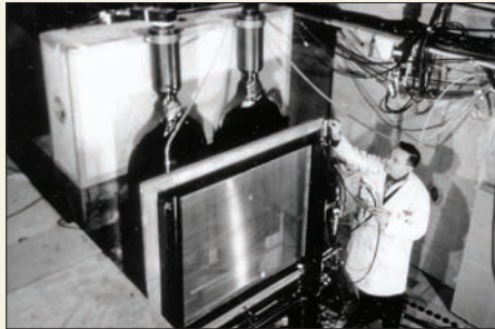
The first wire spark chamber installed in a PS experiment, with scintillation counters behind.
